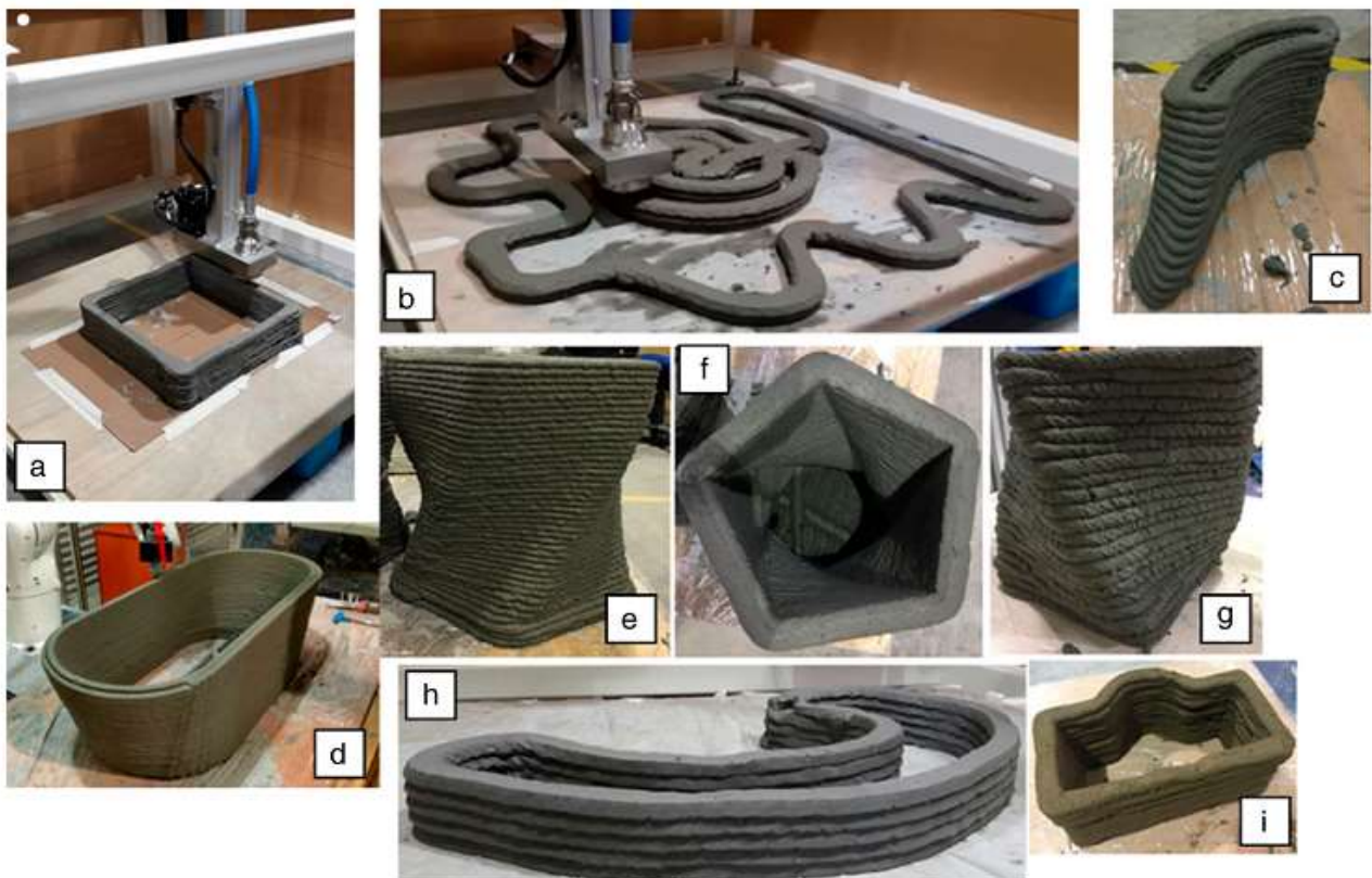
Figure 2: 3D concrete printed objects at SC3DP (prototype) [12]
